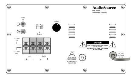
overrides this circuit, turning the subwoofer off manually. The power LED indicates the subwoofer's status.
